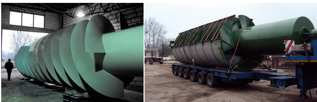
Rys. 10. Stopień wodny Lisi Ogon, transport turbiny Archimedes, Mewat Sp. z o.o. [2, 3]
